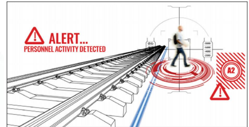
Trespasser detection using a fiber-based sensor device
