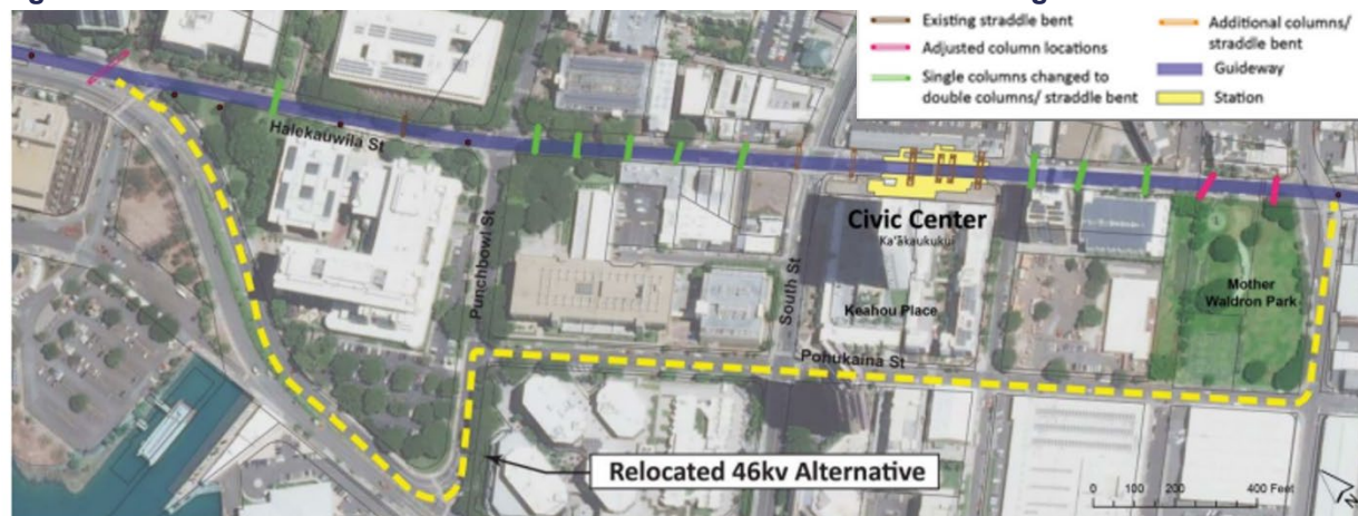
Figure 6. Modification from Center Column to Straddle Bent Column Design on Halekauwila Street
