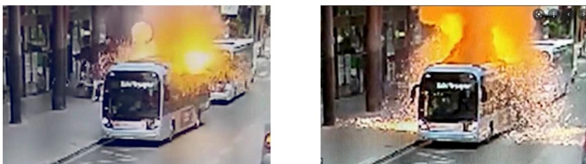
**Figure C-2** Thermal Runaway Images
