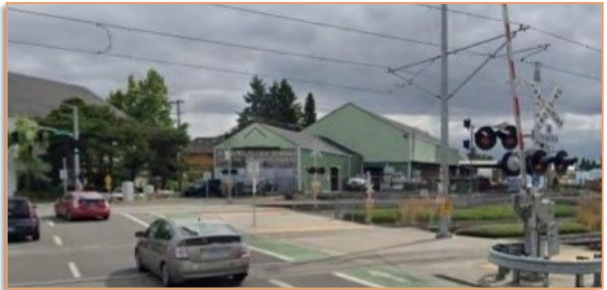
An example of a multi-modal crossing with light rail (foreground) and freight rail (background). Multi-modal crossing configurations are crossings where two or more different types of rail traffic use the same crossing and could be crossing simultaneously under certain conditions.
