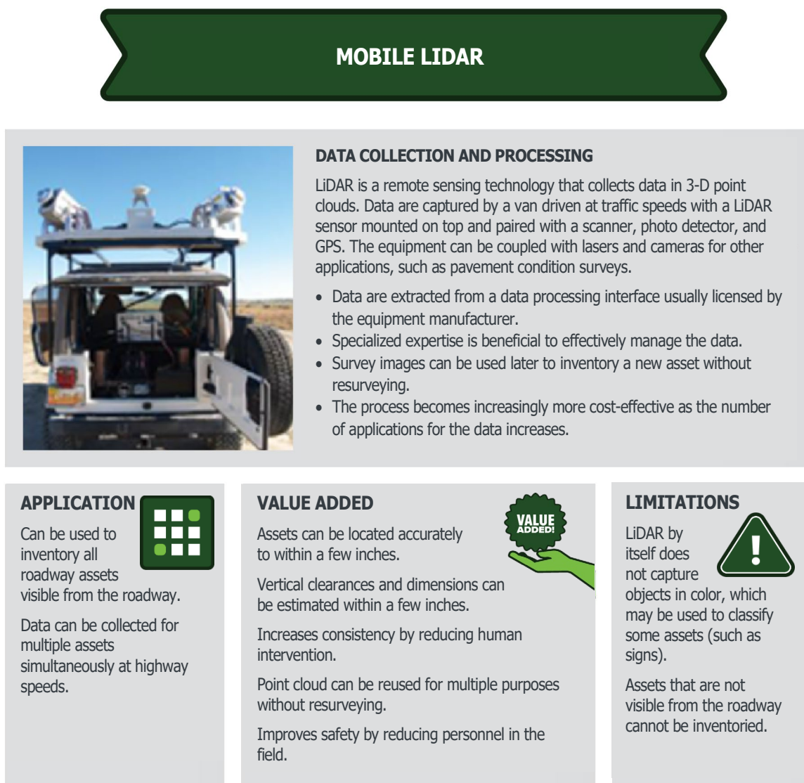
Figure 26. Graphic. Characteristics associated with Mobile-LiDAR data collection techniques (adapted from Zimmerman and Manda 2015 with permission from National Academy of Sciences, courtesy of the National Academies Press, Washington, DC).
