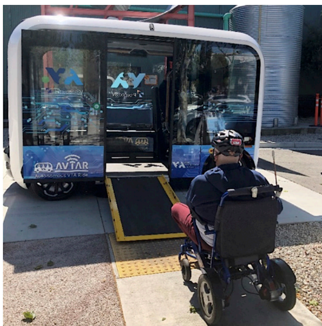
Figure 3-1 Passenger using power wheelchair to board automated Local Motors Olli shuttle
