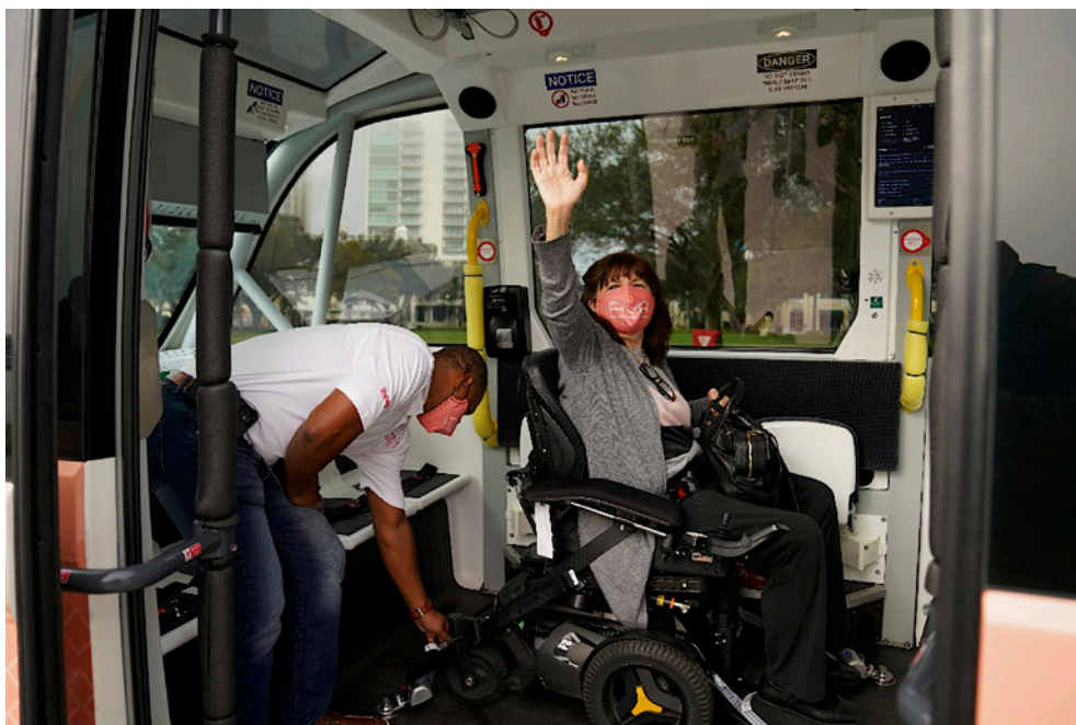
Figure 4-2 Passenger using power wheelchair secured by onboard personnel in Navya automated shuttle
