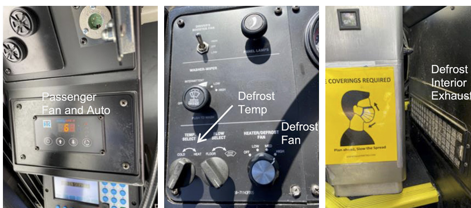
Figure 2-6 Bus C equipped with passenger interior air recirculation (left) and driver defrost interior air recirculation (middle) only; source of exhaust for driver defrost air located on dash panel wall and in front of fare box (right)
