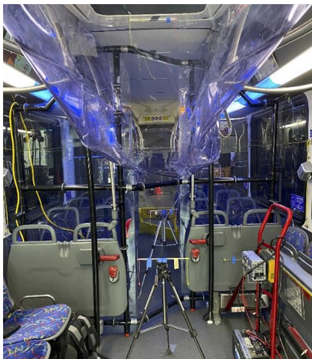
Figure 2-13 Roof exhaust HVAC configuration (bus B) prototype temporary barrier, modified with hood surrounding roof exhaust
