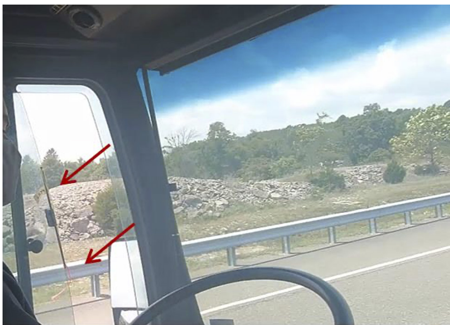
Figure 3-11 Bus B, driver window open and hatches closed, telltales pulled out of window
