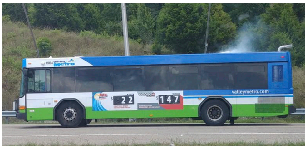
Figure 2-23 VM (bus C) during air flow testing on VSR Highway section; fog visible exiting bus rear roof hatch
