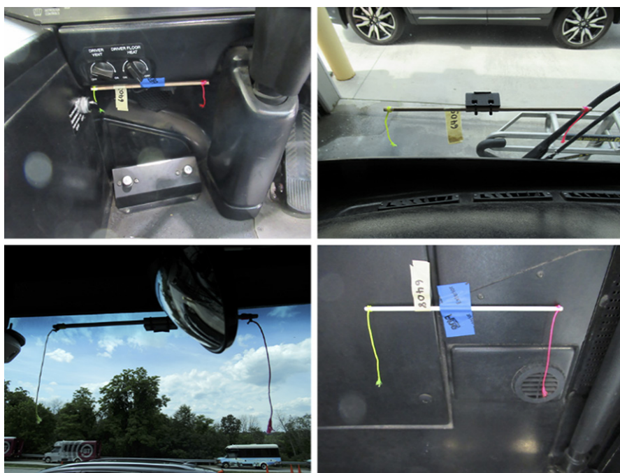
Figure 2-14 Telltale locations near dedicated ducts from driver defrost on bus B—above pedals near steering column (upper left), lower windshield near defrost ducts (upper right), upper windshield (lower left), entry door duct (lower right)
