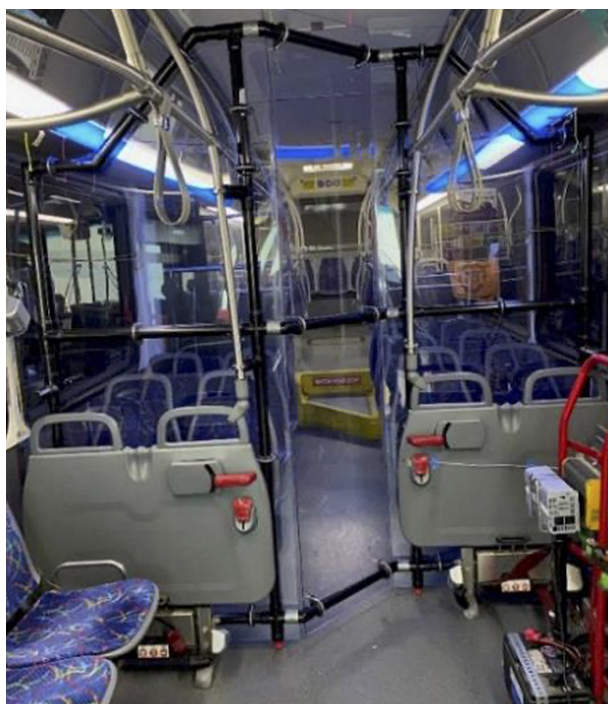
Figure 2-12 Roof exhaust HVAC configuration (bus B) prototype temporary barrier, original with 3-in. ceiling gap on curb side (left) and 1-in. ceiling gap on street side (right)
