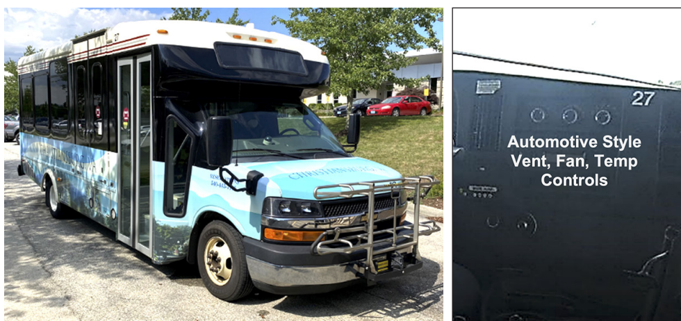
Figure 2-10 BT BoC bus configured with cut-away van driver HVAC and separate roof-mounted rear passenger interior HVAC system
