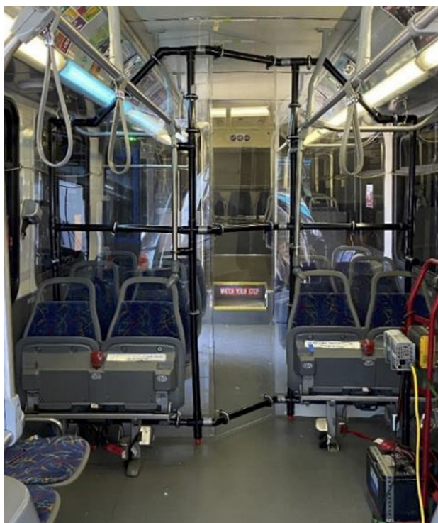
Figure 2-11 Rear exhaust HVAC configuration (bus A) prototype temporary barrier with 3-in. ceiling gap on curb side (left) and 1-in. ceiling gap on street side (right)
