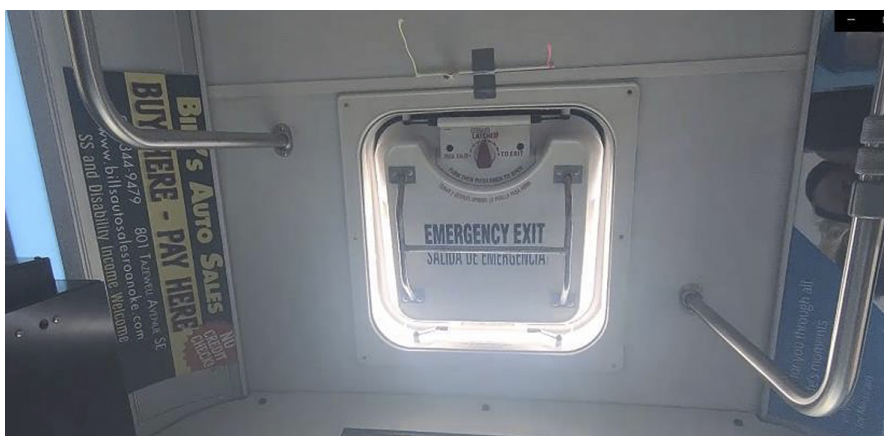
Figure 3-3 Bus C, open front roof hatch near front axle, telltales blowing rearward due to air entering
