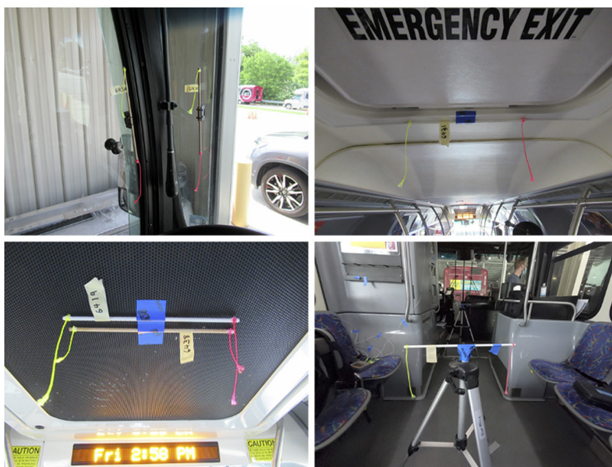
Figure 2-17 Other selected telltale locations on bus B—driver window glass and A-Pillar windshield (upper left), rear roof hatch (upper right), passenger HVAC roof-mounted exhaust (lower left), floor tripods (lower right)
