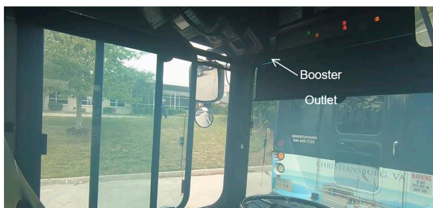
Figure 3-12 Bus C, fog being pulled forward above bus operator workstation with booster fan active
