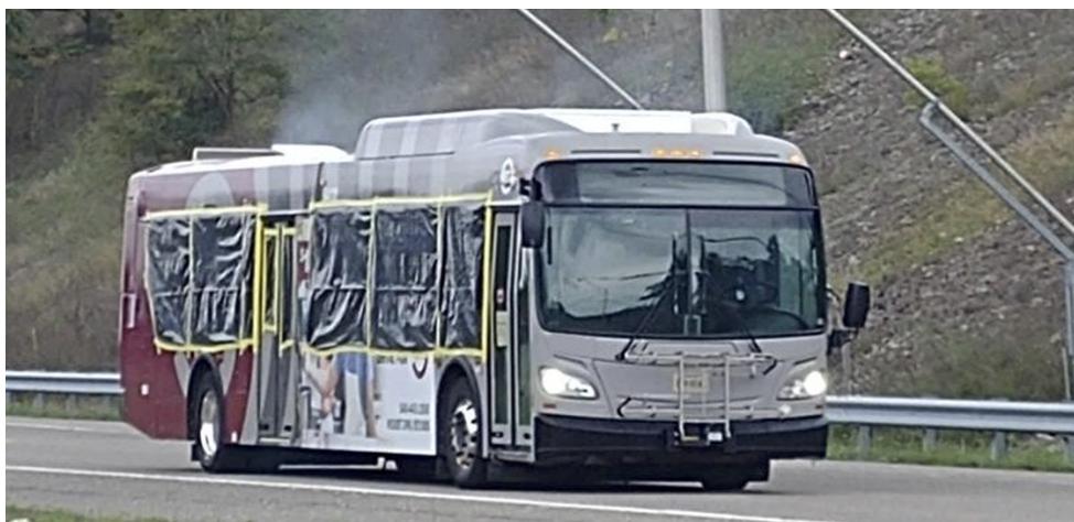
Figure 2-22 BT (bus B) during air flow testing on VSR Highway section; fog visible exiting bus rear roof hatch
