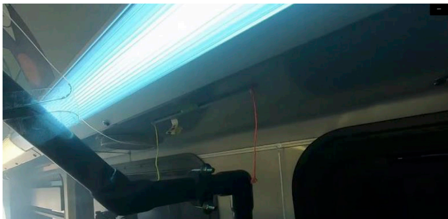
Figure 3-6 Bus A, fog flowing from front to back on curb side of bus with passenger air only
