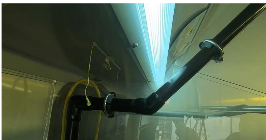
Figure 3-8 Bus A, air shearing fog on back side while bus idling with driver defrost on high with driver window and roof hatches closed
