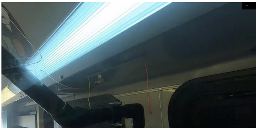
Figure 3-5 Bus A, fog flowing from front to back on curb side of bus with driver defrost air only
