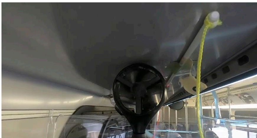
Figure 3-7 Bus A, anemometer demonstration while bus idling with driver defrost and passenger air both on high with driver window and roof hatches closed
