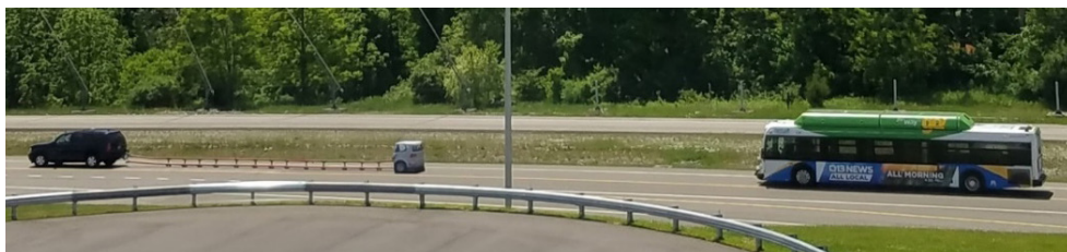
Figure D-4 Forward collision avoidance test
