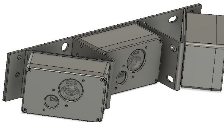
Figure D-1 PASS lidar sensor assembly
