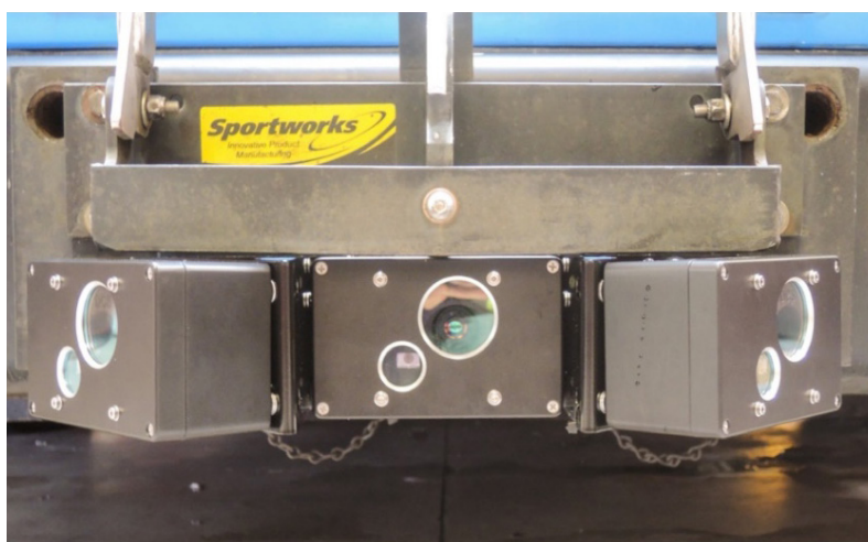
Figure 4-2 PASS sensor array on front of bus
