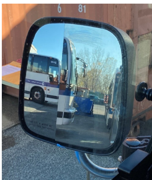
Figure 4-8 Vertical split-glass prototype mirror
