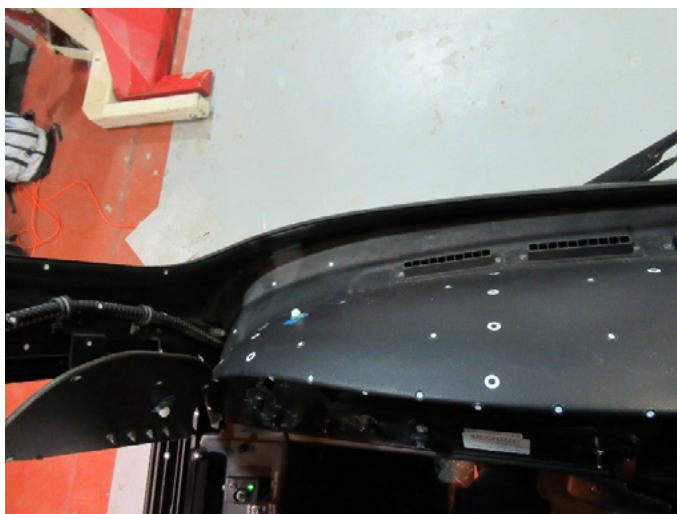
Figure 2-8 Laser scanning photometric and probe reference stickers attached to bus street-side A-pillar and dash
