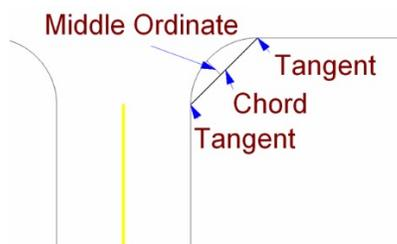
**Figure B-14** Intersection Curve Diagram – Chord Line, Middle Ordinate, and Tangent Points
