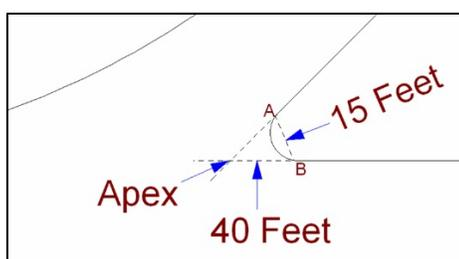
**Figure B-19** *Measuring Intersection Angle – Establish Apex and Mark Off Point along Each Side*
