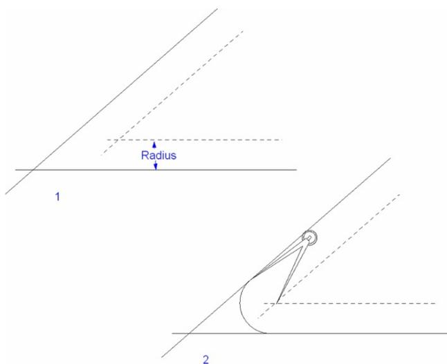
**Figure B-21** Drawing Curve Radius to Scale (Angled Intersection)
