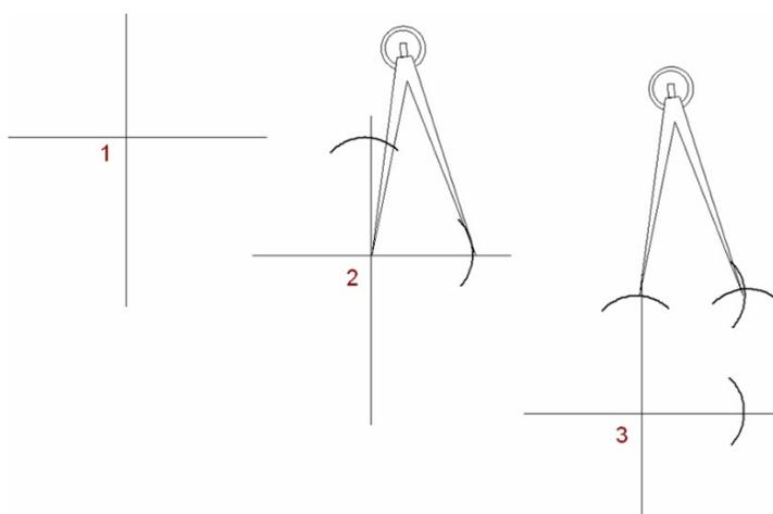
**Figure B-15** Drawing Curves to Scale – Steps 1 through 3 Used in Drawing Intersection Curves to Scale
