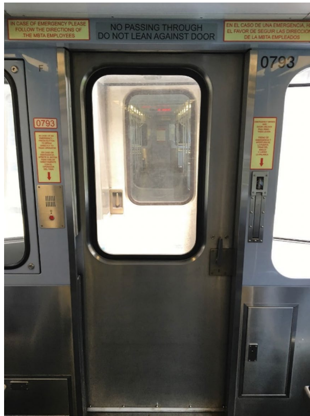
Figure 4-12 End-of-Railcar Door on MBTA Subway Train – Door Locked, includes Signage Instructing Customers How to Unlock Door during Emergencies
