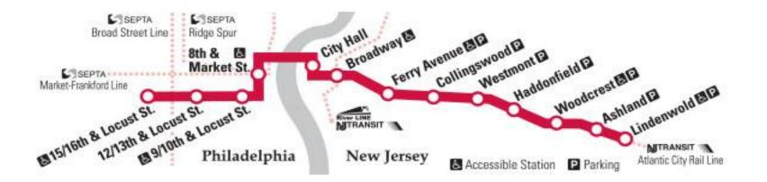
The PATCO line is a double track operation that extends approximately 14.3 miles of double track grade separated system from Lindenwold, New Jersey to the Philadelphia, Pennsylvania and uses the Benjamin Franklin Bridge to provide train service between New Jersey and Pennsylvania.
