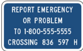
Example of an Emergency Notification Sign (ENS) posted at humped rail grade crossings.
