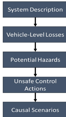
Figure 5-2 STPA method as applied in this study
