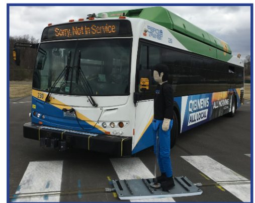
A Pierce Transit bus equipped with the AEB system being tested at the VTTI Smart Road Facility
